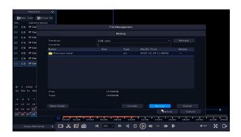
Press "Backup" at this point to record to USB drive You can create new folders if desired for the recording
